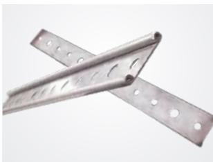
Fastening bars - made from aluminium and magnesium alloy are used to fix waterproofing membrane when changing angles between horizontal and vertical welds and when finishing at the top of the upstand. This can be used to replace the termination and fixing bars. It is highly durable in bending and torsion, as well as resistant to corrosion.
